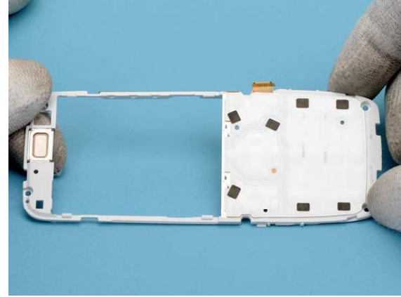
Turn the UI FRAME ASSY over and support the EARPIECE with your fingers to keep it in place.
