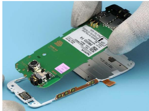
Place the FRAME ASSY under the PWB so that the PWB will not bend while removing the camera.
