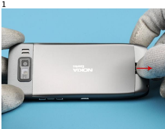
Slide the BATTERY COVER release button to the direction shown in the picture.
